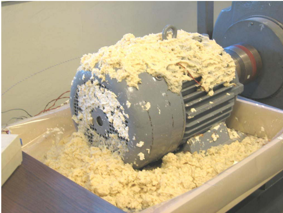
Fig. 6. Motor without cover with pulp spilled over it, and pulp splashed on the air intake area
