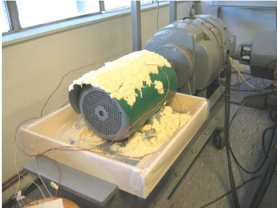
Fig. 9. Motor with pulp spilled over the cover; clean air intake area
